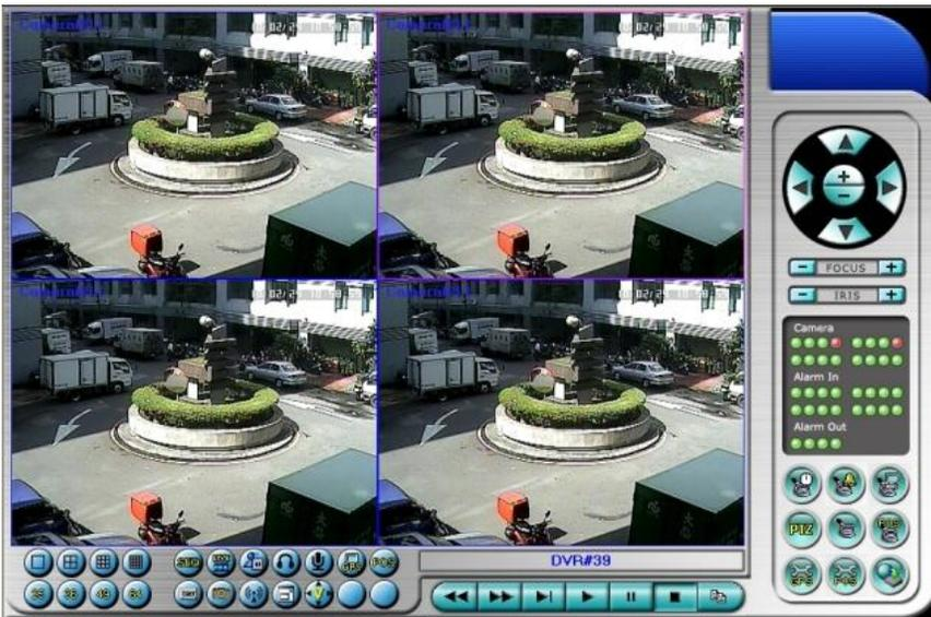
The video images can be displayed in several types of split-window screens, including 1/4/9/16-Window for single DVR and 25/36/49/64 for multiple DVRs. And the focus window is surrounded by a frame border. In addition to the video windows, there are different icons on the lower corner and the right corner of the screen for status display and control. (The “.L” following the camera title stands for Live display, “.P” for Playback, and the camera title with white background has detected motion.)
