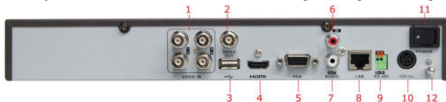
Figure 1.4 Rear Panel of PS-7904SI
