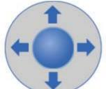
Click to up/down/left/right control movement of the PTZ. When hold on the one direction key, the PTZ will keep circling as that direction after user press the stop
