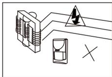
Installation should keep away from high-pressure cable.
